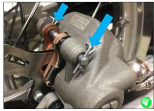
Fig 3. – Correct rear brake mounting
