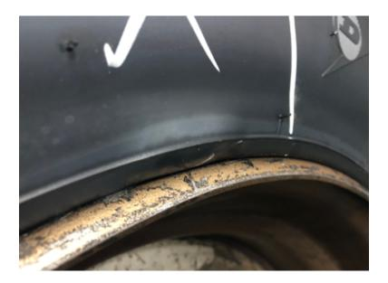
The deformation is to the left of the white line marked on the tire in the photograph. As the photograph shows, this small deformation appears on the surface of the tire near the rim.
