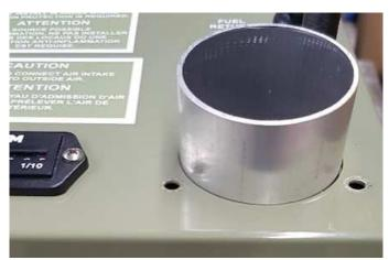
Remove the three screws from the combustion fan intake and pull it down and out to provide better access to the fuel line.
