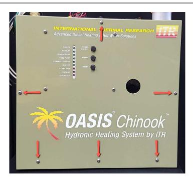
Remove these screws to gain access to the inside of the heater.
