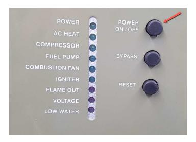
Press the power button and make sure the Power LED has turned off. Wait until the combustion fan turns off. This will take 2-4 minutes.
