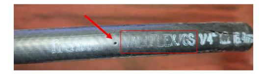
This hose is subject to leaking. If a heater is discovered to have this hose, it must be changed out with the appropriate fuel line as per the instructions below.
