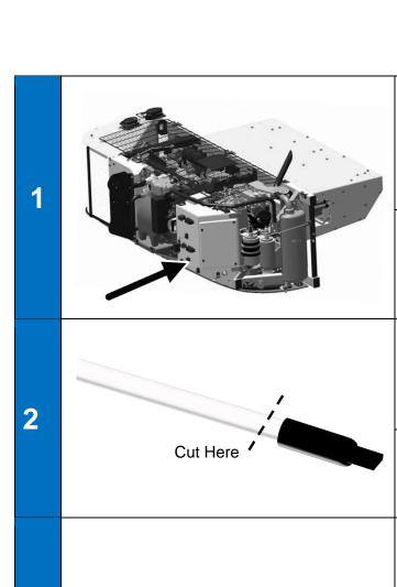
Locate the harness option bundle near the control box
