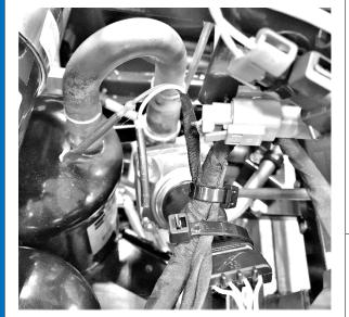
Install heat shrink caps (K) on both of the wires and use heat gun to seal.
