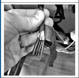
Wrap wire ends together with tape (A1). Continue wrapping tape to end to cover heat shrink.
