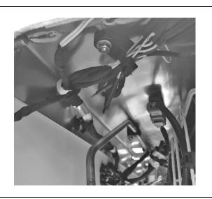
Locate the option bundle in evaporator section.
