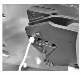
Crimp terminals and seals to the wire. Use the appropriate die position for the size terminal being crimped.
