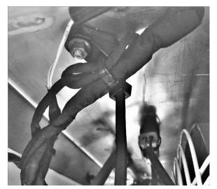
Bundle harness as shown and secure harness with cable tie (J) to cable tie base.
