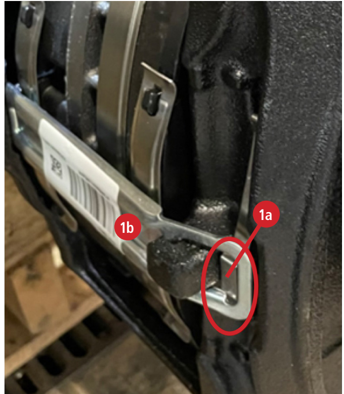
Spring bracket trapped under pad retainer
