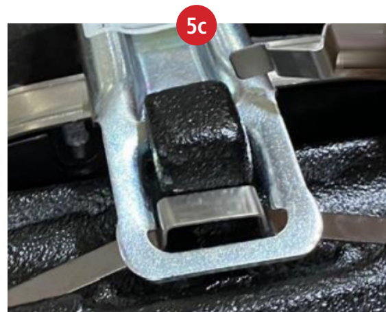
– until spring bracket pops up into its correctly seated position
