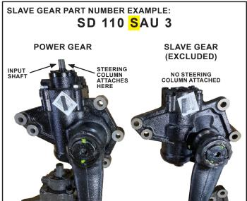
Figure 7 - Slave Gear Part Number and Image Example
