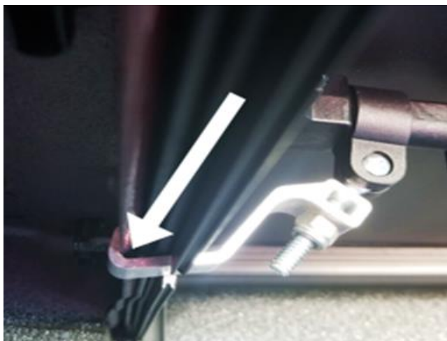
Correct installation of bracket clamp hook
