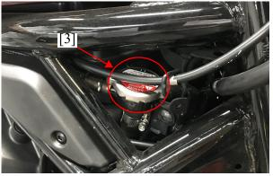
**Note:** Identify the old radiator cap by marking with a permanent marker or scratching an 'X' on top of the cap.
