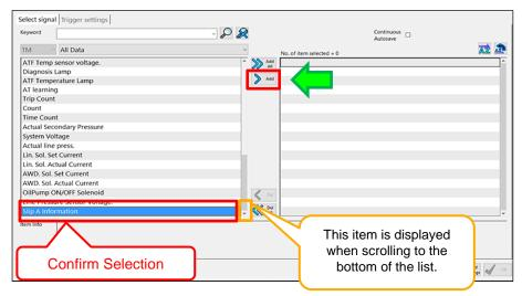
**IMPORTANT:** In the case of failed control module communication with SSM after the installation of the temporary PAK file, check and confirm the interface setting is matched to the equipment being used (SDI, DSTI, & DST 010).
