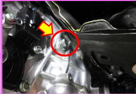
STEP 3C: Install and align the specialty plug / holder (18361AA090) as shown below.
