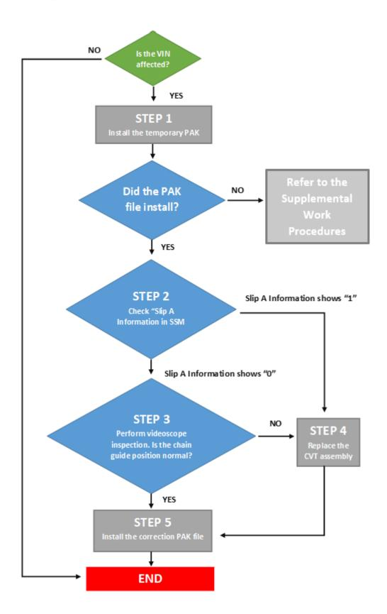
STEP 1-A: Reprogram the Transmission Control Module (TCM) with the TEMPORARY PAK file.
