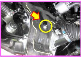
**STEP 3B: CAREFULLY** lift the insulation only as far as necessary to expose the plug as shown below.
