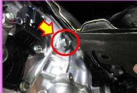
STEP 3C: Install and align the specialty plug / holder (18361AA090) as shown below.
