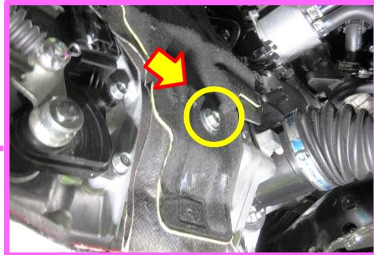
**STEP 8B:** **CAREFULLY** lift the insulation only as far as necessary to expose the plug as shown below.
