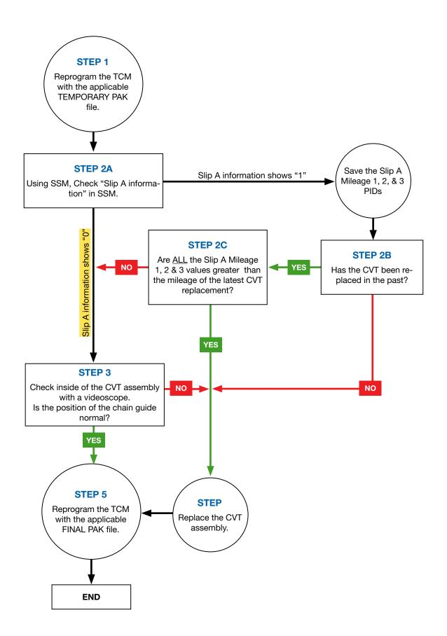
**STEP 1-A:** Perform a DTC check of the TCM and confirm there are no current faults. Any previous faults must be diagnosed, repaired, and cleared prior to reprogramming. Reprogram the Transmission TCM with the **TEMPORARY** PAK file.
