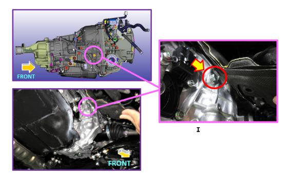
STEP 3C: Install and align the specialty plug / holder (18361AA090) as shown below.
