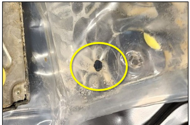
Cover pinched, resulting in puncture.
