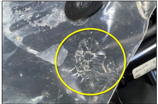
Cover pinched, resulting in puncture.
