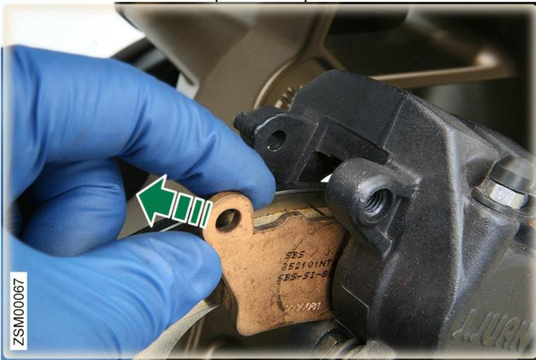
5. Installation of the new brake pads is the reverse of the above removal procedure. When installing the rear brake caliper pin bolt, it should be torqued to 6 ft-lb (8 Nm).
