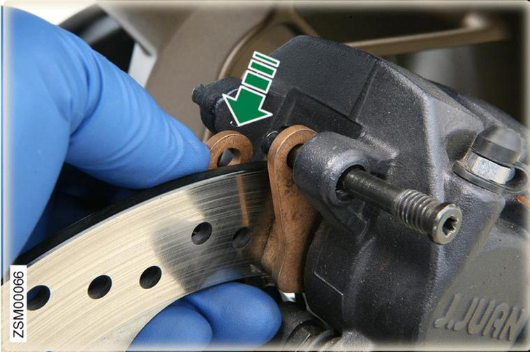
4. Remove both rear caliper brake pads.
