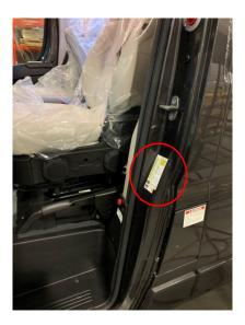
STEP 4: Peel off the backing of the new tire pressure label and apply it over top of the original label with the same orientation.
