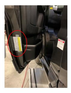
STEP 2: Peel off the backing of the new placard label and apply it over top of the original label with the same orientation
