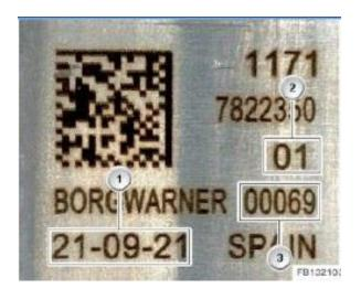
Record or take a photo of the following numbers on the new EGR cooler (1, 2 and 3). These numbers will be required later to register the new cooler in ISTA.
