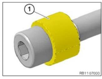
Replace the screws if they do not have the 10mm spacer (1). Use PN 07 14 9 886 429 (included in parts kit 11 71 8 490 650).
