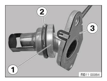
Remove the EGR pipe from the intake venturi pipe (replace O-ring (2) and gasket (3).
