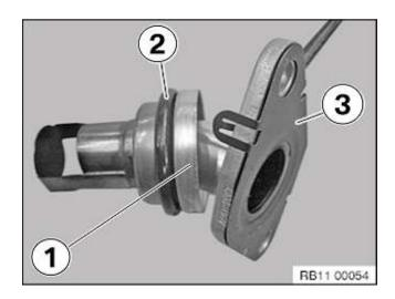
Remove the EGR pipe from the intake venturi pipe (replace O-ring (2) and gasket (3).
