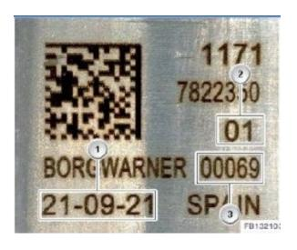
Record or take a photo of the following numbers on the new EGR cooler (1,2 and 3). These numbers will be required later to register the new cooler in ISTA.
