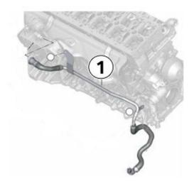
Replace the coolant pipe from the Auxiliary EGR cooler to the coolant pump distribution block (1)
