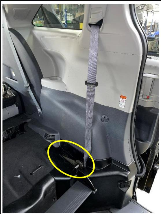
m) Remove the footrest bracket cover by removing two screws
