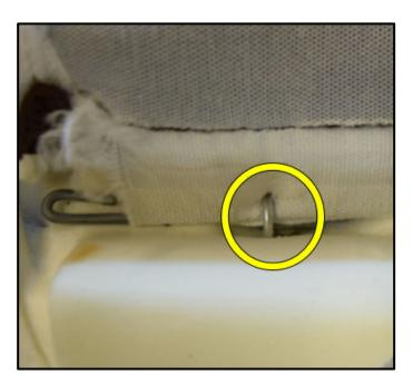
Prior to fully clamping the upholstery clips closed, be sure each upholstery clip engages BOTH the webbing on the bottom side of the seat cover AND the fastening wire molded into the seat cushion as shown <circle>.
