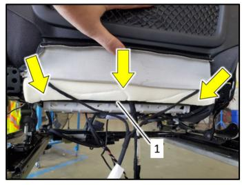
Ensure seat foam <arrows> is fully engaged over the rear of the seat pan <1>.
