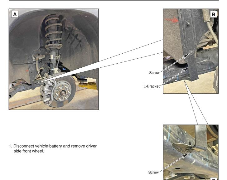
2. Remove wheel well liner L-bracket. See Photos A through C.
