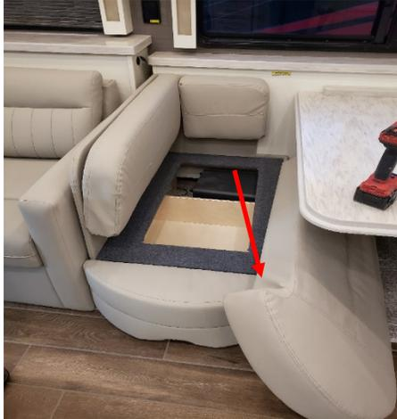
3. Locate the access opening in the cabinet behind the dinette. Using a utility knife, cut a square of paneling off of the main wall in the left corner behind the cabinet access hole.
