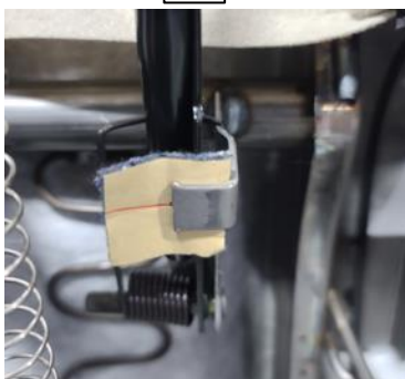
Underside of bracket prior to sticking the felt on permanently
