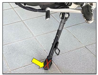
2. Remove the special retaining screw (1) and slide out the side stand switch (2)
