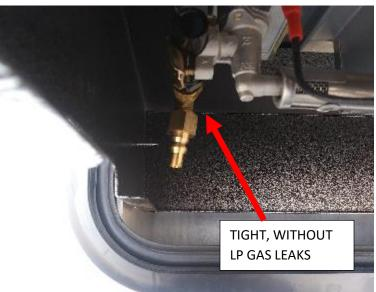
STEP 3: IF THERE IS LEAKING LP GAS, REPAIR THE FITTING;
