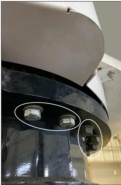
Figure 1 — Outer Race Rotation Bearing Cap Screws and Washers
