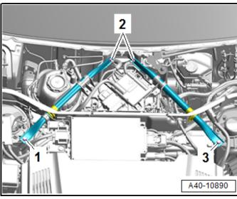
Remove the bolt <3> and nut <2> (left side) and remove the left (driver side) tower brace.
