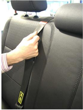
3. Retract the achieved amount of webbing to allow unlocking of the locking mechanism.
