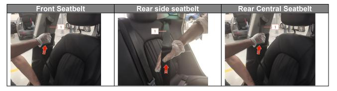
8. Pull on the belt (1) steady and uniformly and verify that it is locked and cannot be pulled out of the seatbelt retractor.
