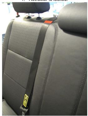
2. Pull out the webbing about 20mm (1 in) with moderate force by hand.
