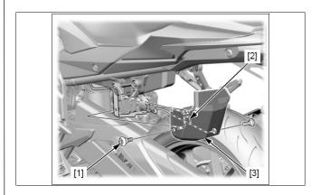
Remove the two bolts [1] from the bottom of the ABS Modulator bracket.
