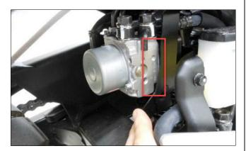
Record the entire lot code and compare it to the table on page two of this service bulletin to determine if the ABS Modulator is Good or No Good. If Good, replace the removed parts and immediately file the appropriate template claim for inspection only. If No Good the ABS Modulator must be replaced.
