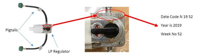
2. File a claim for <u>inspection only</u> if the unit does not have a Winntec model #6020 LP regulator or if the date code stamped into the regulator is <u>not</u> 2017, 2018, 2019 or 2020.
