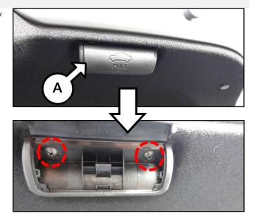
Remove the trunk lid trim by referring to the "Body (Interior and Exterior) → Trunk Lid → Trunk Lid Trim → Repair procedures" in the applicable Shop Manual on KGIS.
