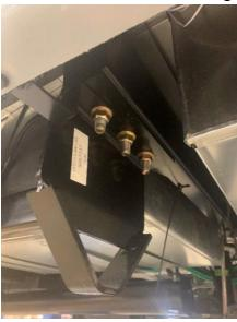
2. On some units, placement of the water tank pan favors one side of the unit. Loosening the tank pan bolts (8) 3/8" hex bolts will allow you to shift the tank and pan slightly aiding in installation of the gusset liners.
