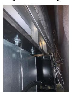
3. Install the gusseted extension liners part # 5125064. Start by feeding the liner gusset inside the gap between the chassis extension and tank pan. Once started, use a mallet or sledge hammer to aid in installing the liner. Using a 2" Grade 8 hex bolt, attach the truss to the liner and extension by feeding the bolt in from the top side and tighten the bolts to 75 ft. lbs. once installed.
