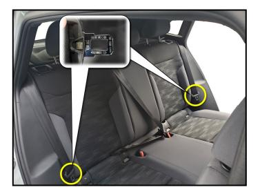
• Inspect both rear outboard seat belts and replace if necessary.
