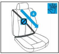
5: Unlatch the seatbelt from the buckle and let it completely retract back into the retractor.
