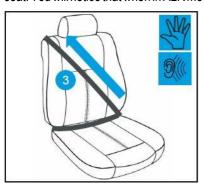
4: Grasp the torso portion of the seatbelt and carefully pull on the belt in an attempt to pull the seatbelt back out of the retractor. The belt should not pull out of the retractor.
