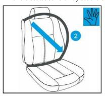
$3: Carefully \ let the \ seat belt \ retract fully into the \ retractor \ while \ the \ belt \ \underline{remains buckled over the \ empty \ seat}, \ this \ simulates \ a \ restrained \ child \ seat. \ You \ will notice \ that \ when \ in \ ALR \ mode, \ there \ is \ a \ ratcheting/clicking \ noise \ from \ the \ retractor, \ this \ is \ normal.$
