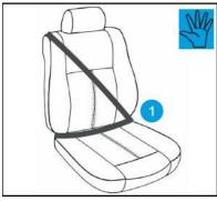
2: Pull the seatbelt all the way out of the retractor to activate the Automatic Locking Retractor (ALR).
