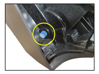
• Re-secure the glove compartment hinge pin.
