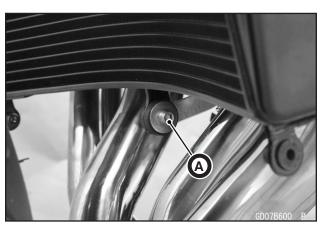
Remove the lower radiator mounting bracket bolt [A] and lower radiator mounting bracket [B].
