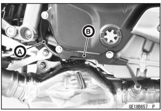
Secure the oxygen sensor lead with clamp [A].
