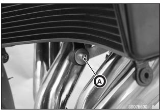
Install the water pipe bolt [A] and tighten to 89 in·lb (1.0 kgf·m, 10 N·m).
