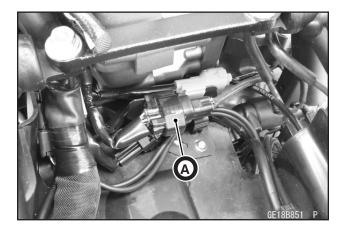
• Free the oxygen sensor lead [B] from the clamps [A].
