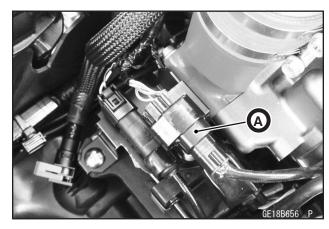
Free the oxygen sensor lead from clamp [A].
