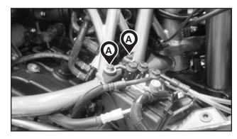
While lifting the ABS hydraulic unit [A], remove the upper radiator mounting bolt [B] (both sides).
