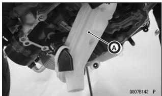
Remove the oil pressure relief valve [A].
