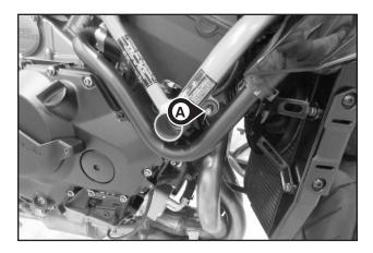
• Remove and retain the lower radiator bolt [A] from the left side of the vehicle.
