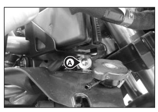
Install the ABS hydraulic unit bracket bolts and tighten to 89 in·lb (1.0 kgf·m, 10 N·m).
