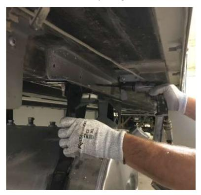
7. Using a combination square, mark a line across the beam in line with the end of the existing tank bracket.
