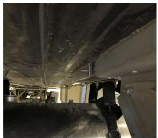
13. Install flat washers and nuts on to the two installed bolts and tighten snug. Repeat these steps for the two remaining inboard bolts. **Note:** Use caution to not overtighten the fasteners or the Composite beam may become damaged.
