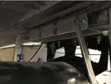
9. Using a Right Angle drill, drill through the beam and out through the previously drilled holes in the existing bracket. **Note:** A 6.5" to 7" bit is optimal for this step.
