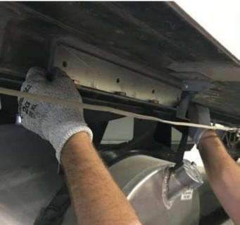
5. Once the Doubler plate is properly positioned, use it as a template to mark the 4 holes for drilling.
