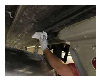
Prep the Composite beam by thoroughly cleaning with paper towel and Accetone or Isopropyl alcohol.
