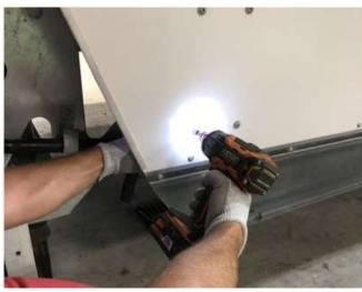
2. Remove the single fastener securing the Safety Tether at the mid-point of the same panel.
