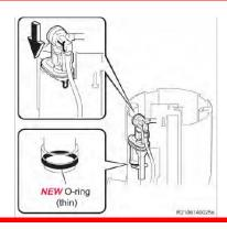
Be sure to apply engine oil to a NEW Oring (thin) and install it to the jet pump.
