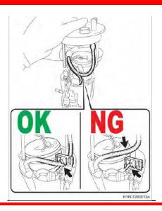
Be sure to pass the 2 fuel hoses under the fuel filter bracket, and be certain to correctly align the upper and lower sections of the fuel suction tube assembly as to not twist the fuel tube.
