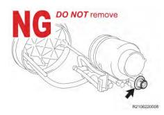
Never remove the fuel pressure regulator assembly from the fuel filter.
