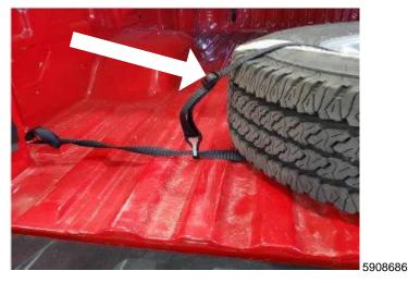
• Tighten both strap buckles to secure the spare tire and wheel assembly.
