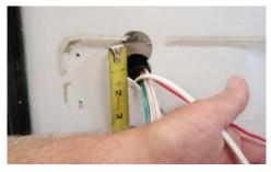
G. DRILL ¾" HOLE BELOW THE TAIL LAMP HOLE A MINIMUM OF 2";
