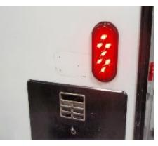
E. INSTALL COSMETIC SNAP RING FOR NEW TAIL LAMP AND CAP SEAL WITH SILICONE.
