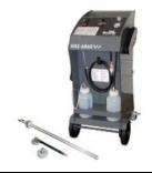
Brake Filling and Bleeding Equipment -VAS6860-(or equivalent)
