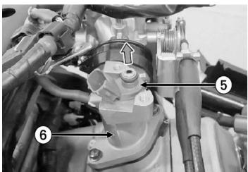
11. Remove the seal ring  $\widehat{\jmath}$  and the O-ring  $\widehat{s}$  from the fuel injector  $\widehat{s}$ .
