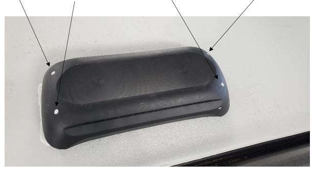
3. Inspect to ensure interior and exterior panels have been routed. If panels have been routed reinstall cover and submit claim for inspect only. (properly routed vent opening)
