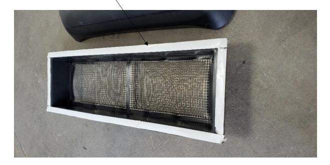
16. Center vent over opening and secure using (16) 1" #8 wood screws. Once you have installed the vent base seal the screws and edge of vent base using self-level sealant.
