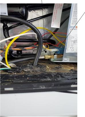
4. Using a flat head screwdriver, disconnect 12v power supply. Tape or wire nut ends of wires to prevent from shorting.
