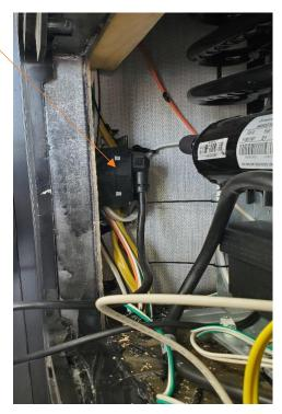
6. Using a square head screwdriver bit and screw gun remove screws from refrigerator base.,
