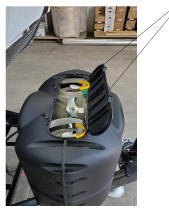
2. Remove cover from lower refrigerator sidewall vent by twisting locks so that the slots are in the vertical position.  $\sim$
