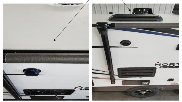
2. If vent is installed, remove top cover by removing 4 screws one in each corner,
