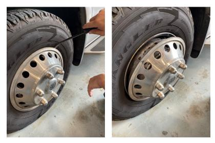
2. Inspect the valve stems for any signs of damage or wear due to contact with the wheel liner. If damage is found, please contact Wayfarer warranty department at 205-487-4710.
