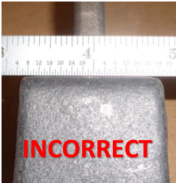
INCORRECT LOCKING MECHANISM INTERNAL LOCK IS STRAIGHT
