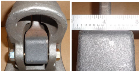
INCORRECT LOCKING MECHANISM INTERNAL LOCK IS STRAIGHT
