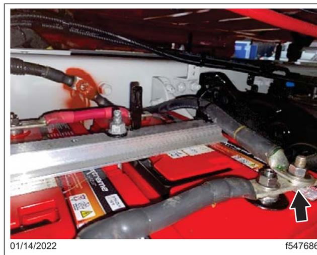
**Fig. 31, Negative Battery Cable Connection at the Battery Post**
