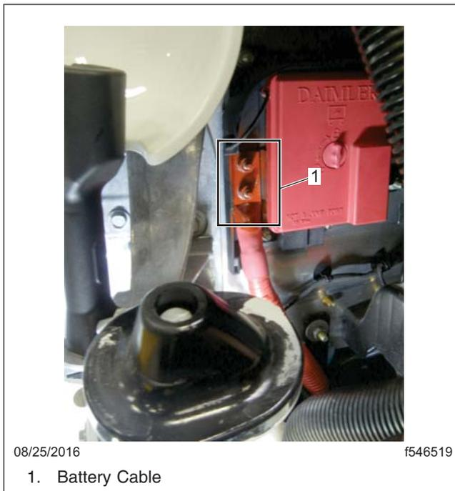
**Fig. 38, BCA Battery Cable (Engine-Side Frontwall)**
