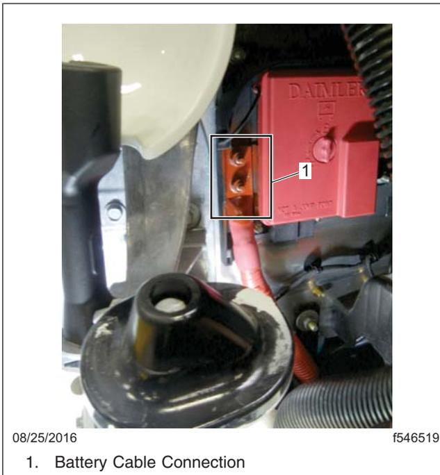
**Fig. 9, BCA Battery Cable (Engine-Side Frontwall)**
