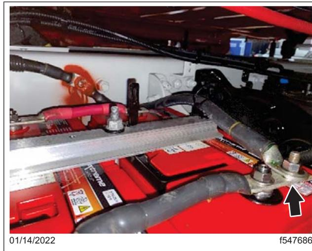
**Fig. 22, Negative Battery Cable Connection at the Battery Post**
