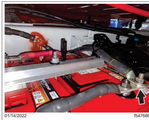
**Fig. 28, Negative Battery Cable Connection at the Battery Post**
