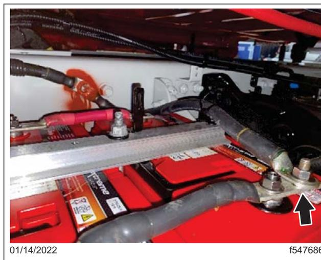
**Fig. 33, Negative Battery Cable Connection at the Battery Post**
