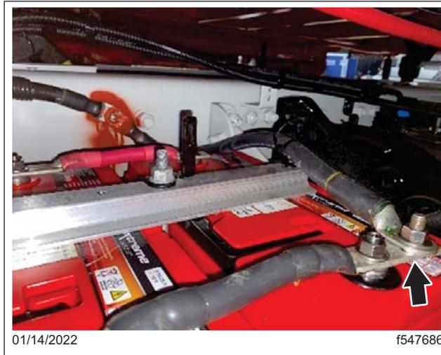
**Fig. 20, Negative Battery Cable Connection at the Battery Post**
