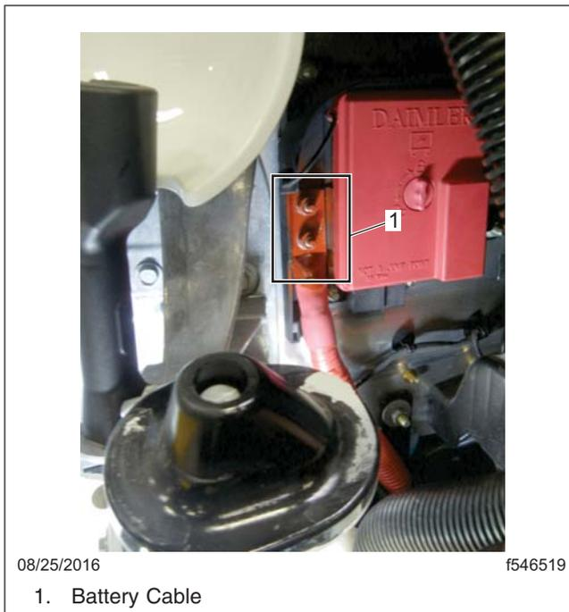
**Fig. 38, BCA Battery Cable (Engine-Side Frontwall)**
