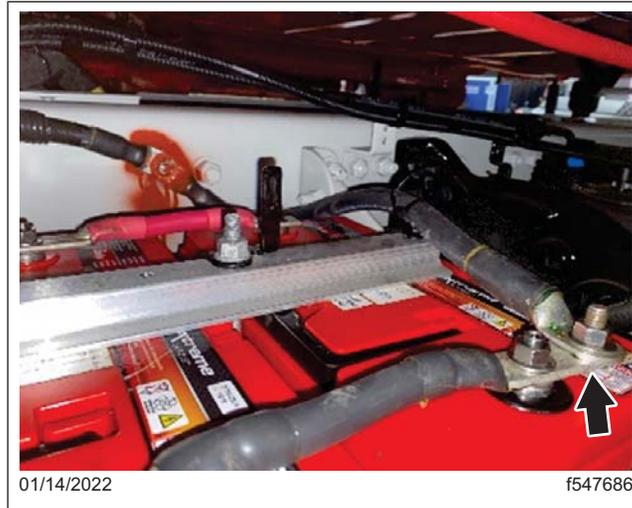
**Fig. 6, Negative Battery Cable Connection at the Battery Post**
