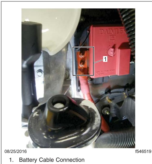
**Fig. 24, BCA Battery Cable (Engine-Side Frontwall)**
