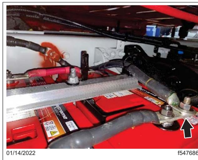
**Fig. 15, Negative Battery Cable Connection at the Battery Post**
