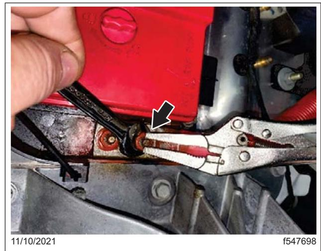
**Fig. 25, Holding the BCA Stud**
