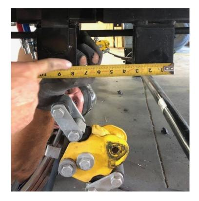
Step 5: Using the center marks to locate the new hangers, clamp all hangers in place on the frame. Verify that the hanger spacing is 29.5" center to center. Use the holes in the hangers to match drill the frame rails with a 3/8" drill bit and drill bit stop.
