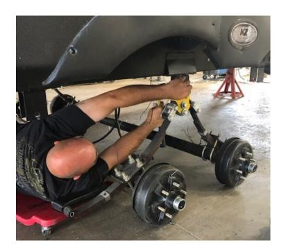
**Step 1:** Remove fender skirt and skirt metal from axle area.
