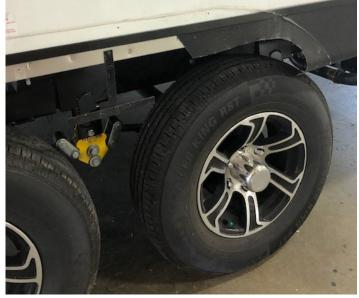
**Step 11:** Test fit fender skirt to new axle location. Mark outer profile with grease pencil on unit. Verify that previous holes will be covered by fender skirt. Holes that will not be covered will need body repair and covered by the amber reflector.
