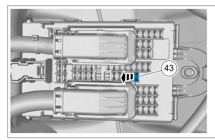
Remove the fuse for the fuel pump (FP).
