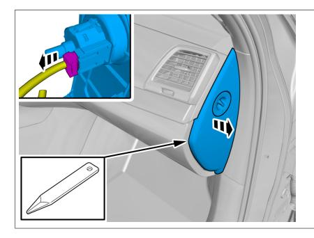
Disconnect the connector. Remove the marked part.
